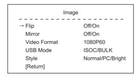
Flip: Enable/disable the picture up/down flip Mirror: Enable/disable the picture left/right flip
